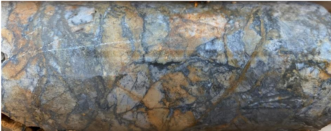
Figure 2: DDH22-045@38.3 m – Altered Quartz Vein & Volcanic Fragment Breccia – in 17.75 gpt Au/1.25 m
