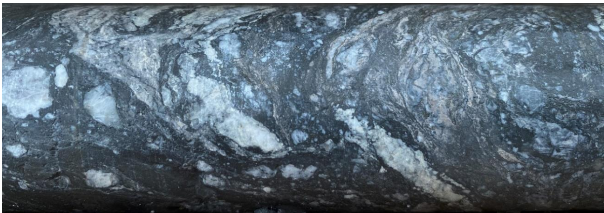
Figure 4: DDH22-045@116.35 m – Quartz & Ankerite Vein Fragment Breccia near "037 Vein" – in 2.87 gpt Au/2.0 m
