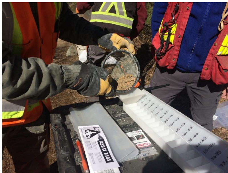
Left: Collecting the reference drill chip trays from the RC drilling at Reliance.
