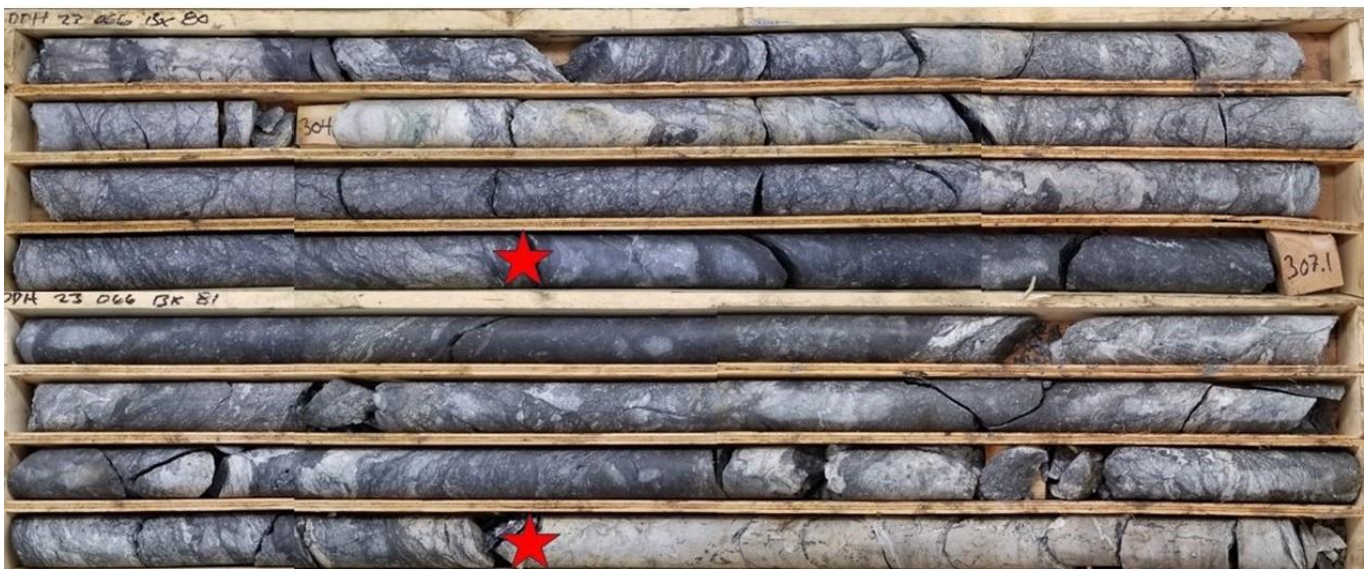
Figure 2 – Reliance Imperial Zone DDH23-066 upper 4 m interval. DDH23-066 - 4 m intersection of Imperial Zone mineralized cataclastite breccia at 306.5 m
