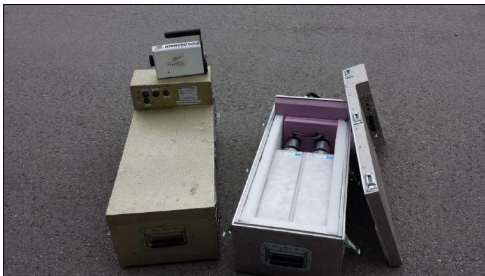
Figure 10: GRS-10 thallium-activated sodium iodide gamma spectrometer crystal packs. The open unit on the right shows two individual 4.2 litre gamma detectors.
