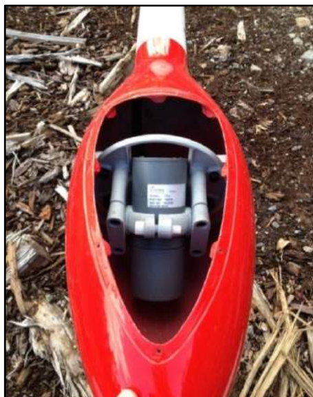
Figure 9: View of “stinger” configuration. Cesium vapor magnetometer sensor orientated 45° from vertical to couple with local magnetic field.
