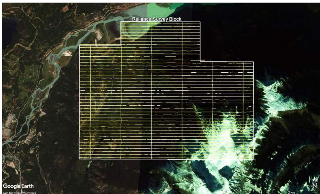
Figure 3: Plan View – Reliance survey block with actual flight lines in yellow and survey block boundary in white.
