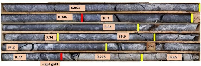
Figure 4: Reliance Imperial Zone DDH23-066 – Detail of High grade Cataclastite Breccia
